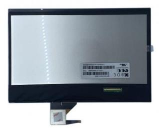
ZH101IP33025V.C is a color active matrix TFT LCD module using amorphous silicon TFT's (Thin Film Transistors) as an active switching devices. This module has a 10.07 inch diagonally measured active area with WXGA resolutions (1280 horizontal by 800 vertical pixel array). Each pixel is divided into RED, GREEN, BLUE dots which are arranged in vertical stripe and this module can display 16.7M colors. The TFT-LCD panel used for this module is adapted for a low reflection and higher color type.
