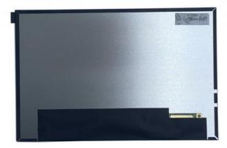
LJ101WXM isacoloractivematrix TFTLCDMDLusingamorphous silicon TFT's (ThinFilmTransistors) as an active switching devices. This module has a 10.1 inchdiagonally measured active area with WXGA resolutions (1280 horizontal by 800 vertical pixel array). Each pixel is divided into RED, GREEN, BLUE dots which are arranged invertical stripe and this module can display 16.7 M colors.
